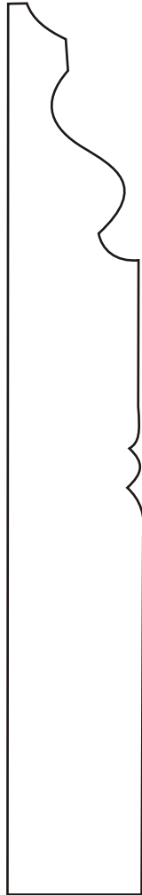
PA224-S 3/4 X 5-1/4 BASE 3/4 X 5-3/16 (MEASURED)
