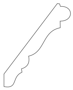
MW030-s 7/8 x 5-1/4 Crown 3/4 x 4-3/16(measured)
