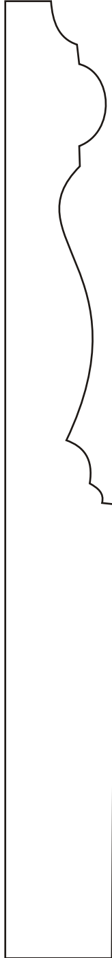
ht227-s 3/4 x 7-1/4 base 7/8 x 7-1/4 (measured)
